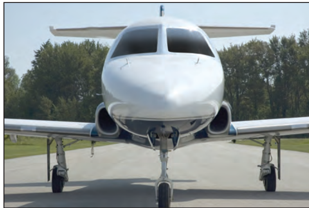
D-JETS/N003—sporting a new paint scheme—viewed from straight-on, to illustrate the windshield and surrounding structure designed to Part 23 bird strike criteria.
