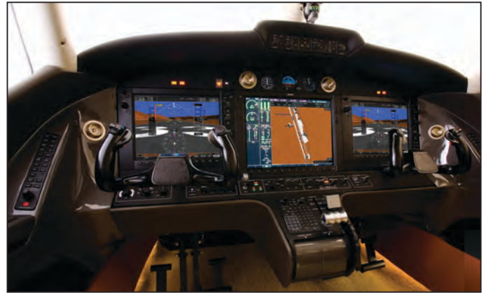
The D-JET's Garmin G1000 glass cockpit.
