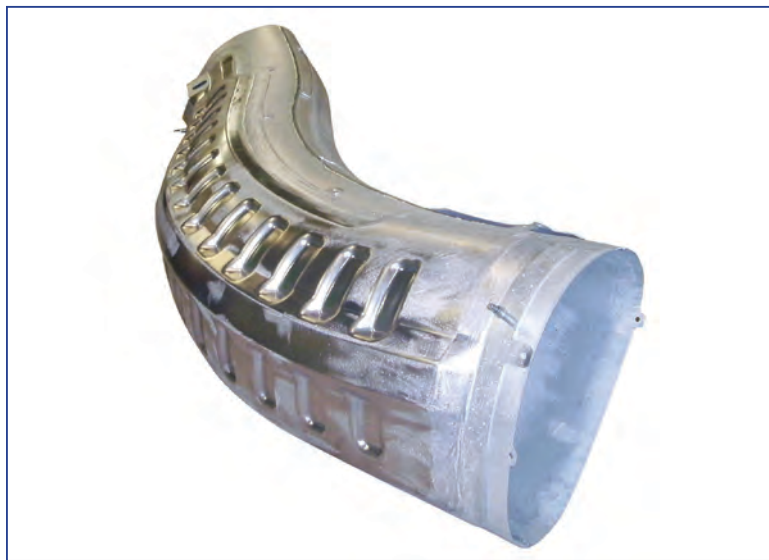
First production certification air inlet duct, for S/N 004.
